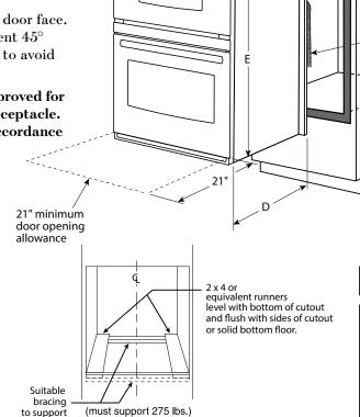
Cutout depth Cutout width 28-1/2" MIN. 28-5/8" MAX. (Junction box may be located Cutout height 42-3/16" MIN. 42-1/4" MAX. Recommended minimum cutout location from the floor 21-5/8" 30"
