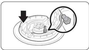
2. Install the burner head so that the electrode passes through the opening for the electrode. Make sure the burner head lies flat on the stove top.
