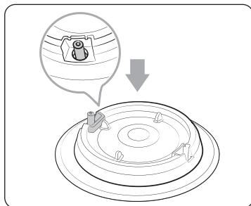
2. Install the burner head so that the electrode passes through the opening for the electrode. Make sure the burner head lies flat on the stove top.
