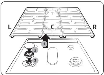
1. Remove the center burner grate(C) following both sides grates.(L/R)
