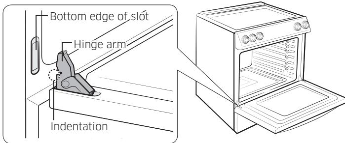
3. Open the door fully. If the door will not open fully, the indentations are not inserted correctly in the bottom edges of each slot.
