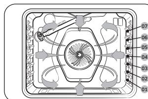
The convection fan at the back of the oven circulates hot air evenly throughout the oven cavity so that food is evenly cooked and browned in less time than with regular heat.
