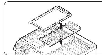
The griddle can be used only with the center burner on the center grate. Use caution when putting the griddle on the center grate.
