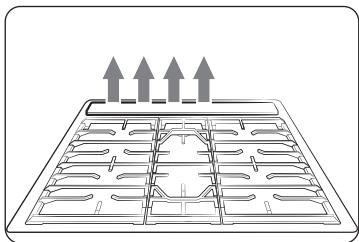
The Oven/Cooling vents are located at the back of the oven range. Proper air circulation prevents combustion problems and ensures good performance.
