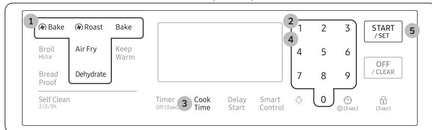
1. Press the pad corresponding to a desired cooking mode such as **Bake**.
