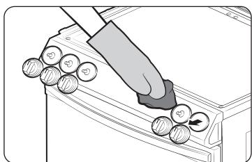
1. Pull knobs off the control valve stems.
