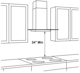
The vent hood must be installed 24" min. above the cooking surface. For optimal performance, install hood more than 36" above the cooking surface is not recommended. The hood installation height abo cooking surface depends upon ceiling height. The telescopic duct cover conceals the ductwork runnii the ton of the hood to the ceiling.
