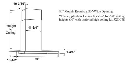
The vent hood must be installed 24" min. and 36" max. above the cooking surface. The hood installation height above the cooking surface depends upon ceiling height. The telescopic duct cover conceals the ductwork running from the top of the hood to the ceiling.
