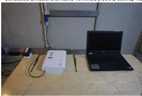
Radiated Emissions (30MHz-1GHz) Test Setup
