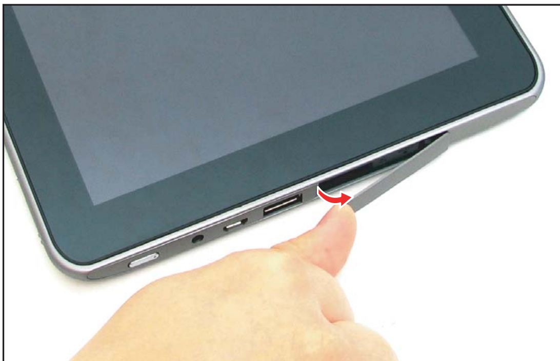
Figure 5-7. Opening the SD Card Cover
