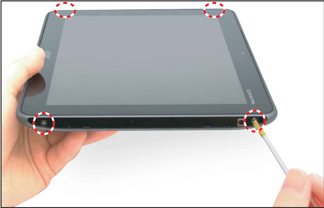
Figure 5-23. Installing the Lower Case (4 of 4)
