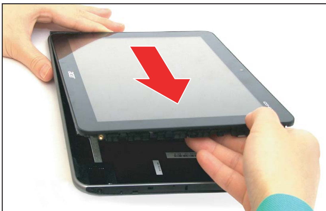
Figure 5-18. Releasing the Side Latches (4 of 4)
