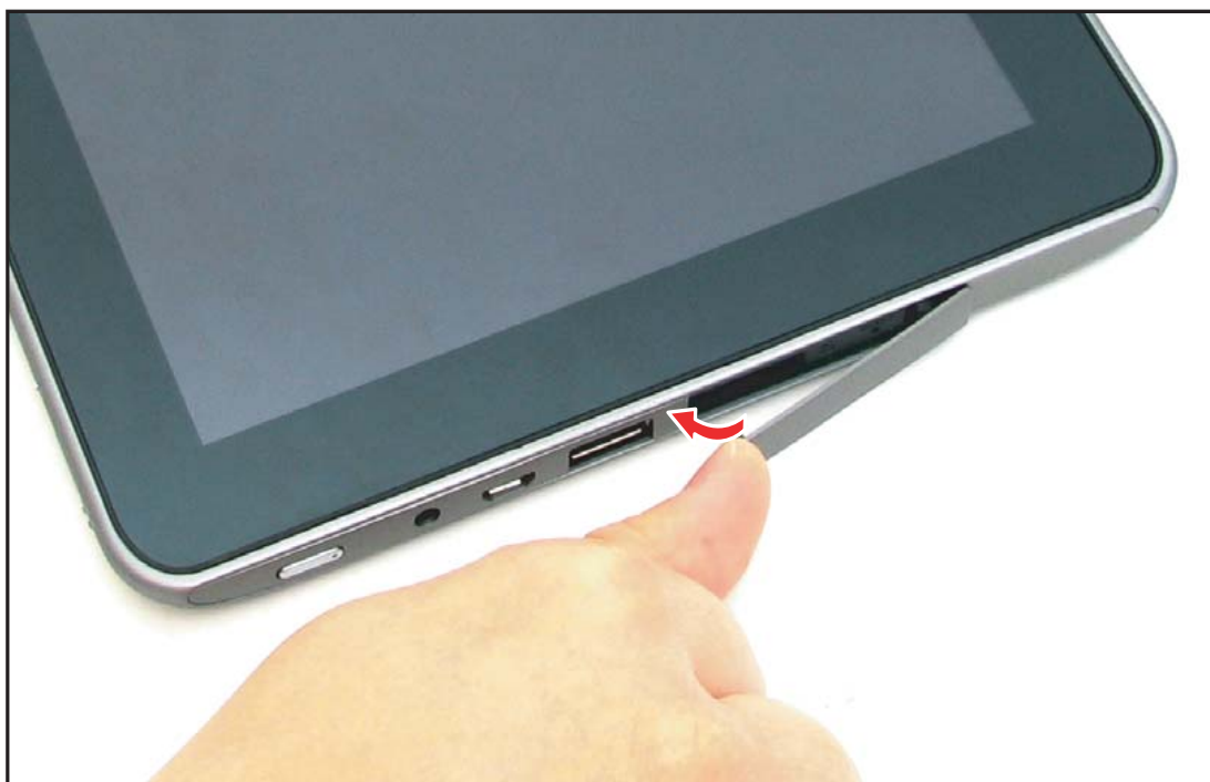
Figure 5-5. Securing the SD Card Cover
