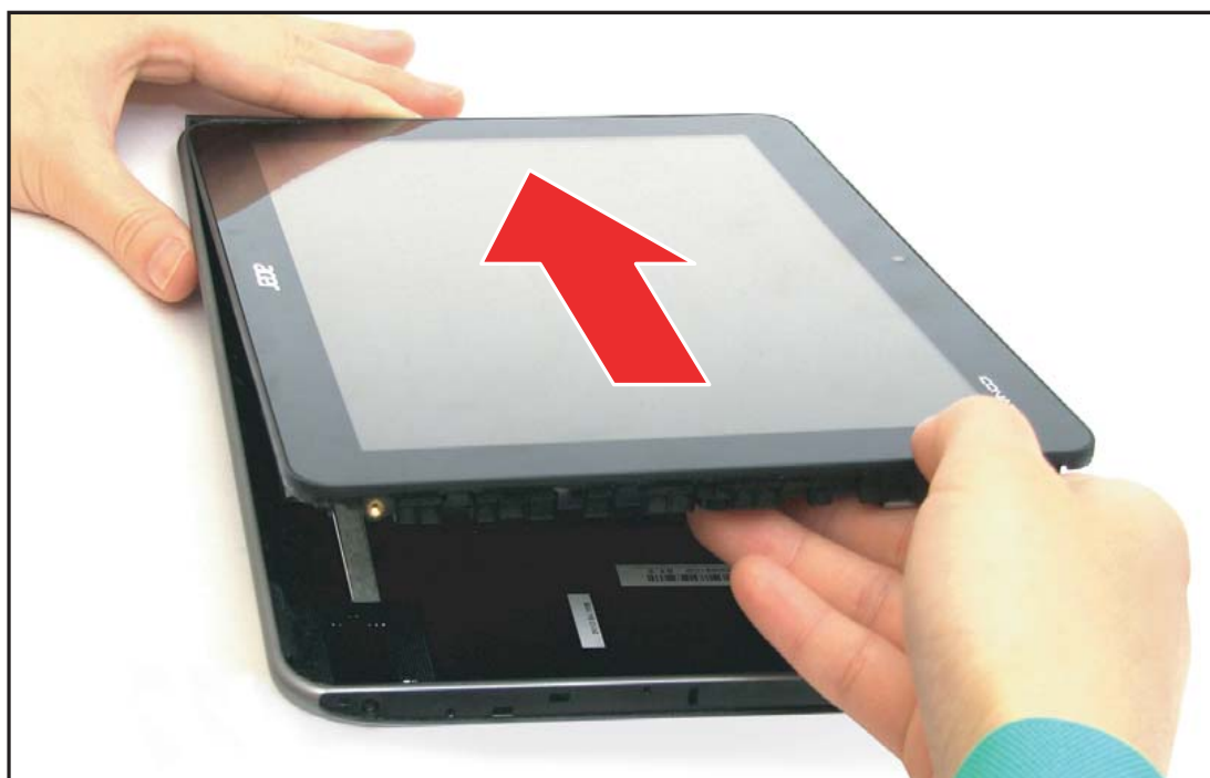
Figure 5-20. Installing the Lower Case (1 of 4)
