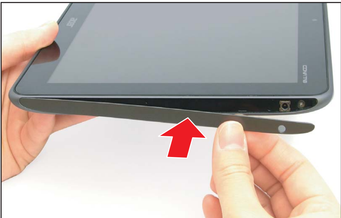
Figure 5-24. Installing the Right IO Cover
