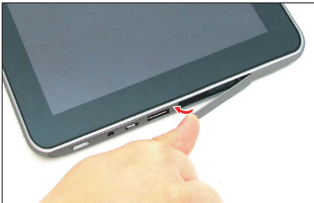
Figure 5-27. Closing the SD Card Cover
