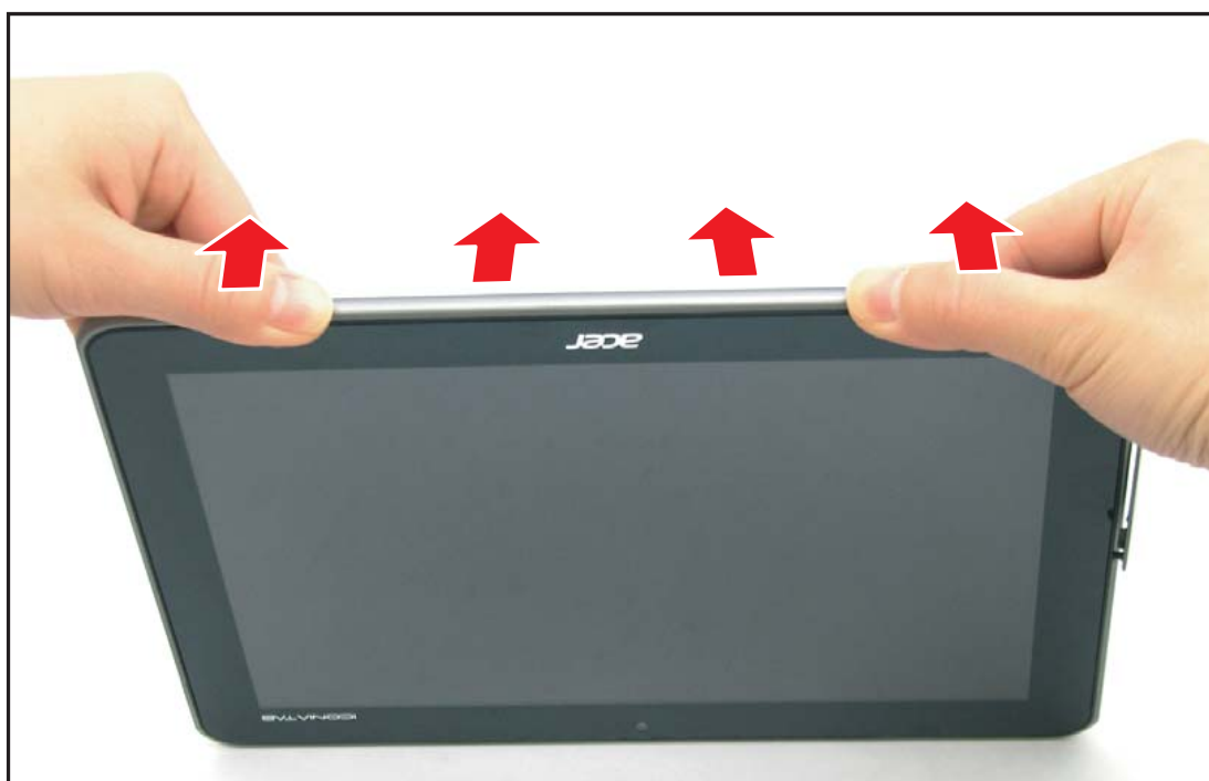
Figure 5-16. Releasing the Side Latches (2 of 4)
