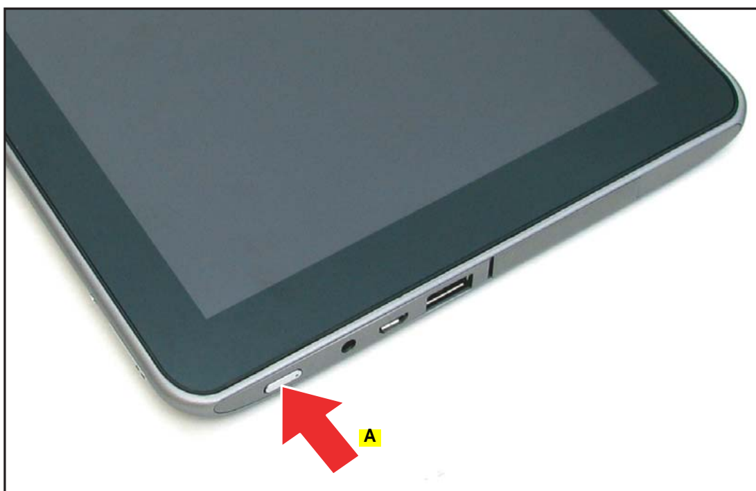
Figure 5-2. Device Overview with Power Button
