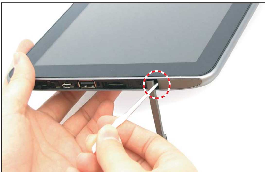
Figure 5-10. Unlocking the Left IO Cover Latches (3 of 4)
