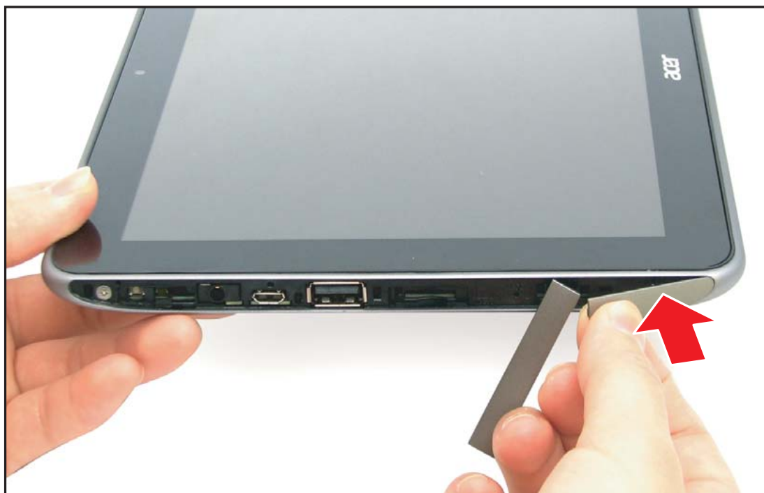
Figure 5-25. Installing the Left IO Cover (1 of 2)
