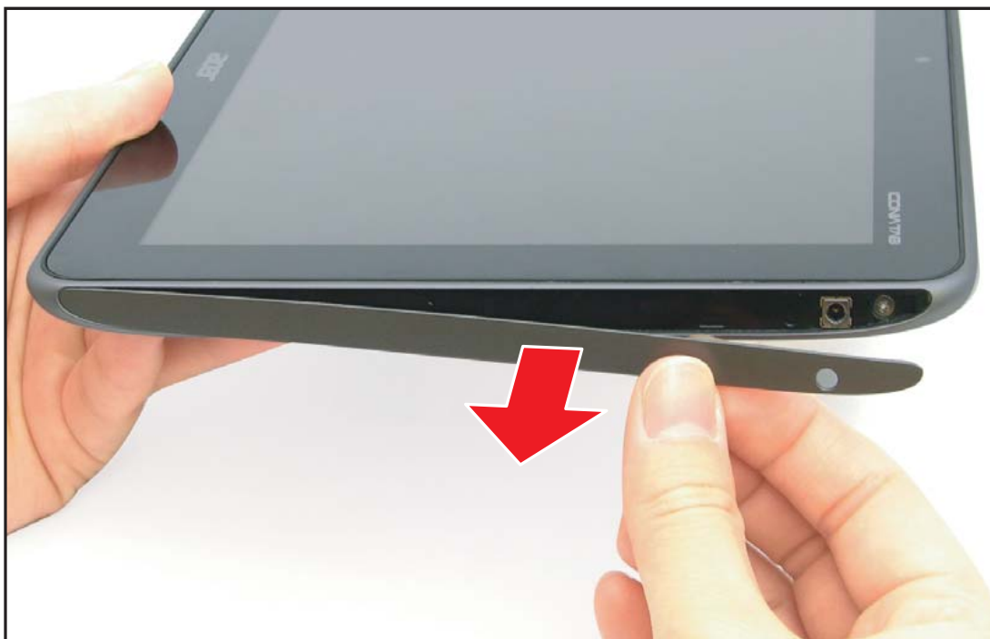
Figure 5-13. Unlocking the Right IO Cover Latches (2 of 2)
