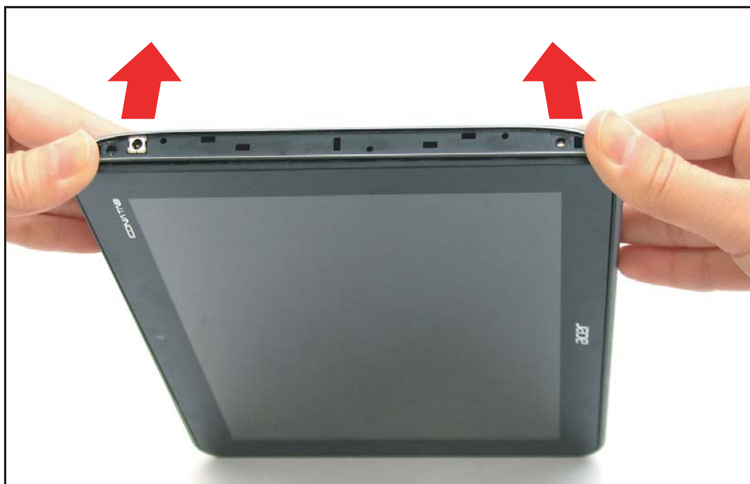
Figure 5-17. Releasing the Side Latches (3 of 4)
