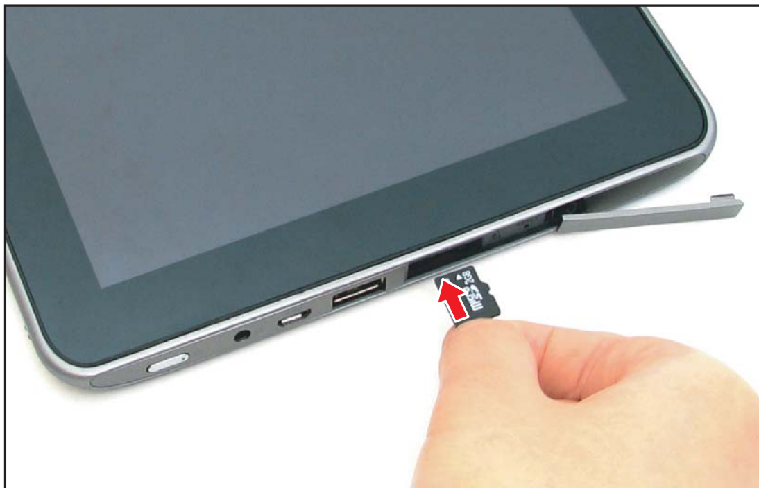
Figure 5-6. Installing the SD Card
