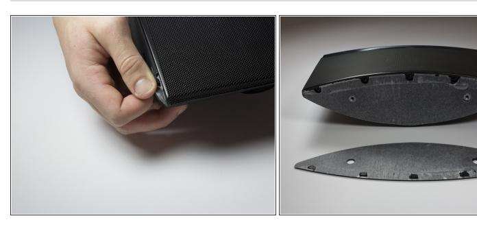
• Use a spudger or your fingers to pry off and remove the rubber pad on the bottom of the speaker.
