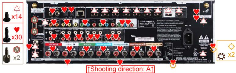
(2) Remove the connector PCB.
