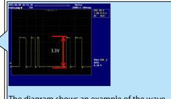
The diagram shows an example of the waveform of pin 129. (I2SO Data)
