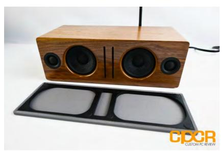
Up front, the Audioengine B2 uses a magnetic grille. Removing the grill, we can see that there's two 2.75" Kevlar woven glass aramid composite woofers with rubber surrounds along with two 3/4" ferro fluid cooled silk dome tweeters with neodymium magnets. At the very center there are two ports in the center for an increased bass response.
