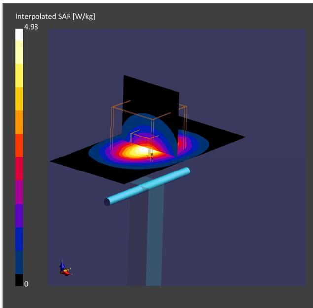
**6. System Check Body Liquid 5300MHz**
