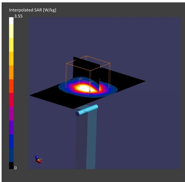
**8. System Check Body Liquid 5600MHz**
