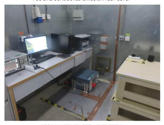
FCC RADIATED EMISSION TEST SETUP
