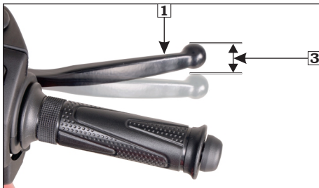
(1) Front brake lever (3) Free play: 10-20 mm
