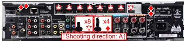
(2) Remove the connector PCB.
