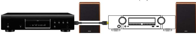
※ In order to check, connect the player to the HDMI terminal and configure the player as AVR source. Check the sound output while turning on the player.
