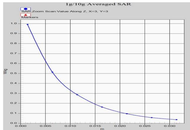
Fig. 1-3 Z-Scan at power reference point (WCDMA1900 Body)
