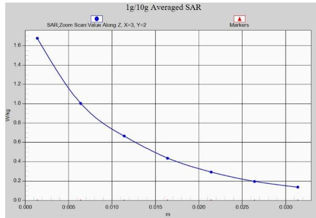
Fig. 1-1 Z-Scan at power reference point (850 MHz Body)
