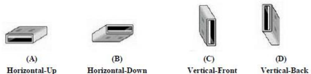
Note: These are USB connector orientations on laptop computers; USB dongles have the reverse configuration for plugging into the corresponding laptop computers.
