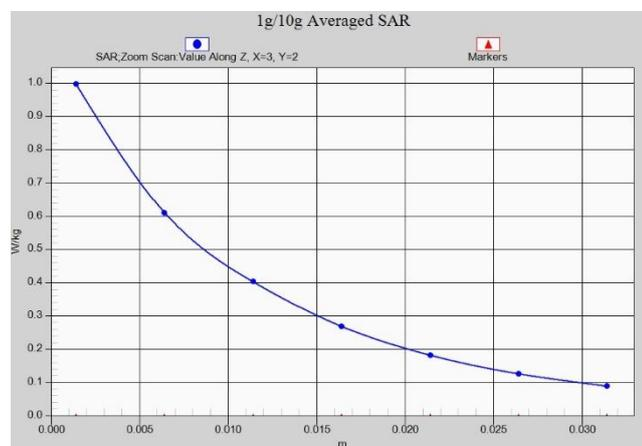
Fig. 1-5 Z-Scan at power reference point (WCDMA850 Body)
