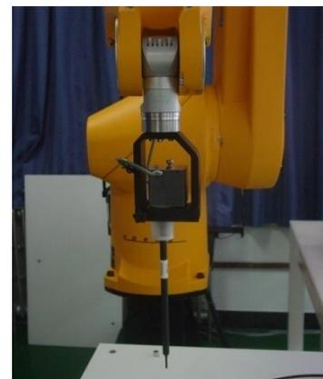
Picture C.3E-field Probe
