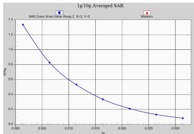
Fig. 1-2 Z-Scan at power reference point (1900 MHz Body)
