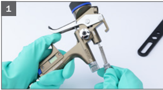
1 First remove paint needle.
