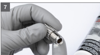
7 Grease thread of material flow control screw
