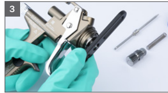
3 And finally, unscrew fluid tip with the ring spanner integrated in the universal spanner.
