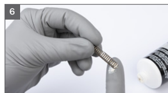
6 Grease and insert paint needle spring
