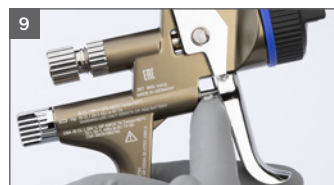
9 Grease visible part of air piston rod
