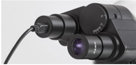
Eyepiece camera fixed into the tube
