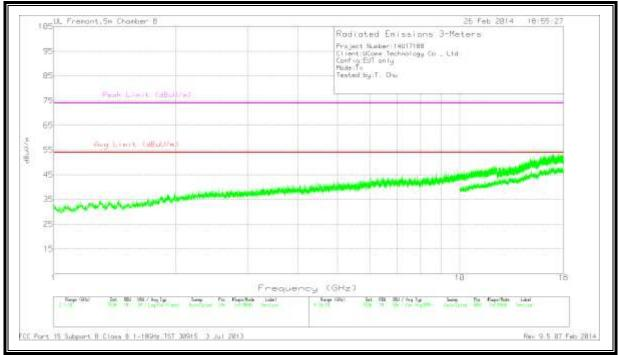
NOTE: there are no emissions found from EUT above the system noise floor level from 1GHz to 18GHz.
