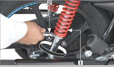
(1) Rear shock absorber (A) Stiffer (2) Pin spanner (B) Softer
