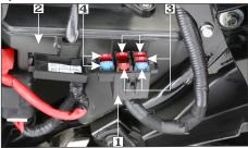
(1) Fuse box (2) Air cleaner assembly (3) In circuit fuse: 15A, 10A, 10A, 10A & 10A (4) Spare fuse: 15A & 10A
