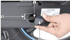
(1) Drive chain (3) Drive chain slack: 30 mm (2) Hole cap
