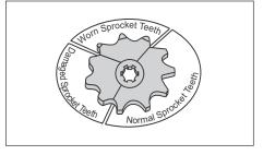
• If the drive chain or sprockets are excessively worn or damaged, they should be replaced. Never use a new chain with worn out sprockets since this will result in rapid chain wear.
