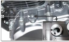
(6) Timing hole cap with O-ring (7) 'T' mark (8) Index mark
