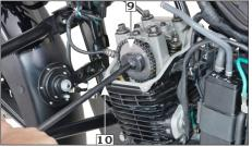
(9) Cam sprocket (10) Special tool
