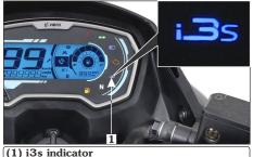
**Initial activation of the i3s system:** Keep the i3s switch (2) to "ON" position. Turn the ignition key to "ON" position. The i3s indicator on the speedometer console will glow for 2 seconds and turn "OFF". Start the vehicle (in neutral and clutch lever released condition) with less than 2000 r/min and let it idle till engine temperature reaches more than 75°C. The engine will cut-off in 30 seconds.
