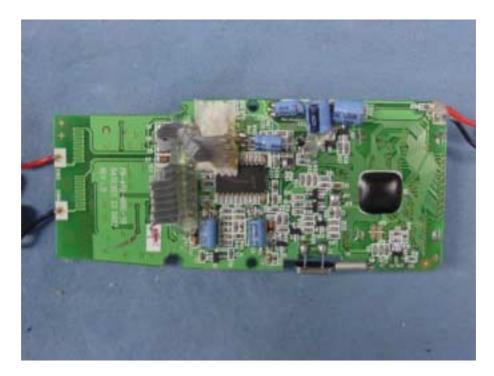
Figure 22 Main Board, Component Side
