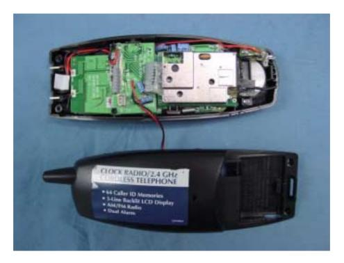
Figure 9 Main Board, Component Side
