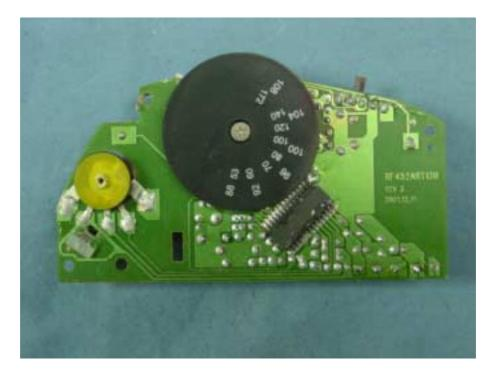
Figure 11 Main Board, Component Side
