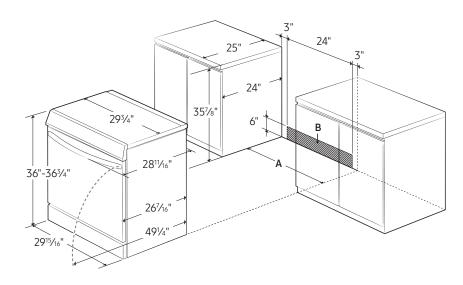
A: Cabinet opening min 30" B: Acceptable electrical outlet area
