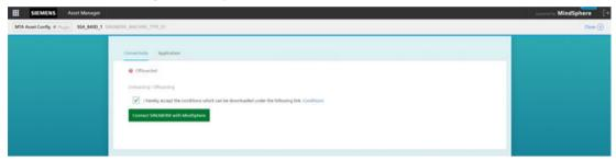
5. Then press "Connect SINUMERIK with MindSphere" to onboard the Machine.
