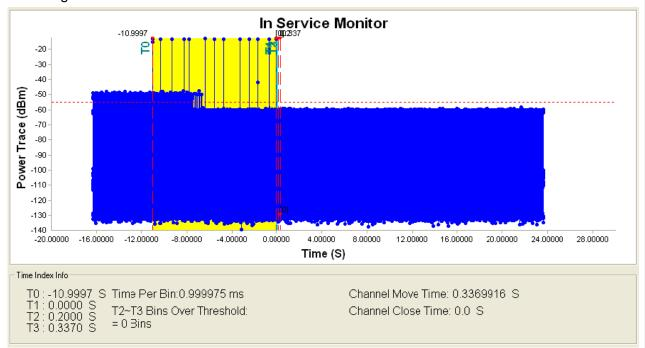
Note: T0 denotes the start of Channel Move Time upon the end of the last Radar burst.
