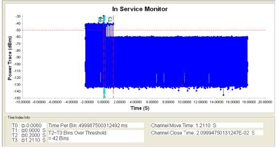
**Note:** To denotes the start of Channel Move Time upon the end of the last Radar burst.
