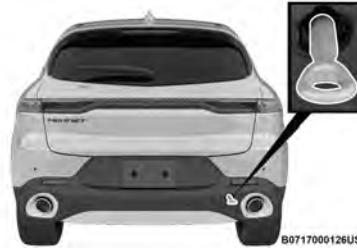
Rear Tow Eye Installed
