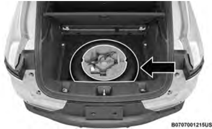
Damaged Tire Storage
