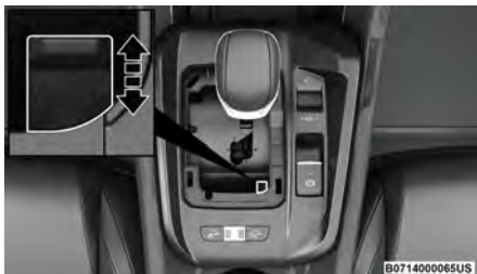
Gear Selector Override Access Location
