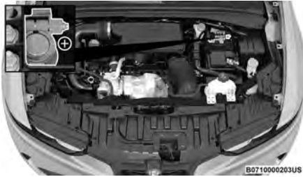
Positive (+) Battery Post
