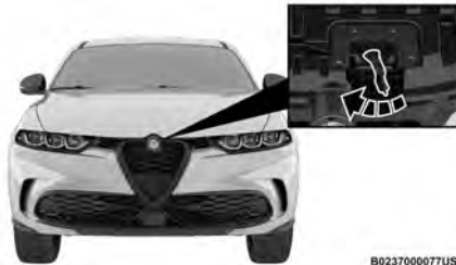
Hood Safety Latch Release Lever Location
