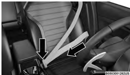
Inserting Latch Plate Into Buckle
