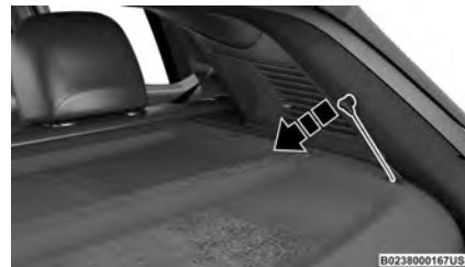
Disconnect Rear Shelf Support Links
