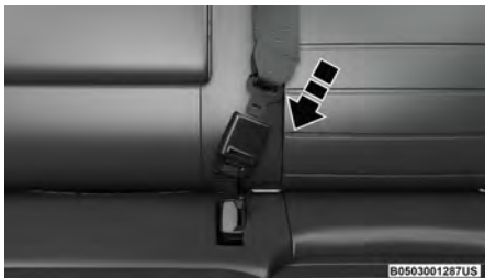
Inserting Mini-Latch Plate Into Mini-Buckle
