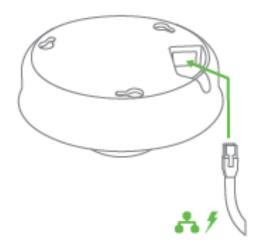
4. Mount the camera to the mount plate guide pins and turn clockwise and then remove the protective bubble cover.
