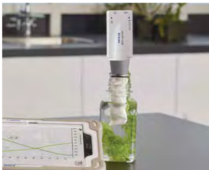
CO 2 Sensor shown in use with Dissolved CO 2 Waterproof Sleeve.
