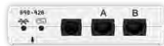
Wireless and rechargeable, the //control. Node has two ports for stepper motors, two ports for servo motors, and one port for digital sensors.
