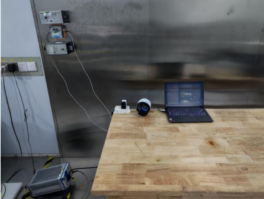
Conducted Emissions at AC Power Line (150kHz-30MHz)
