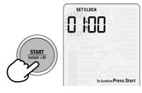
Minutes now flash to show they can be adjusted. Turn TIME dial to adjust minutes and press START button to confirm.
