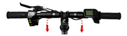
4. Fold the handlebar by gently pulling the 2 spring-loaded clasps apart, using a gentle pulling force to release, then fold the 2 handles away
