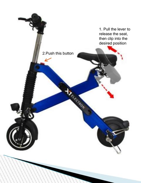
3. To fold or unfold, simply squeeze the bike into the open or folded position after you have positioned the seat correctly
