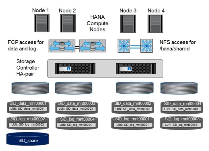
For each SAP HANA host, a data volume and a log volume are created. The <code>/hana/shared</code> volume is used by all hosts of the SAP HANA system. The following table shows an example configuration for a 4+1 multiple-host SAP HANA system.
