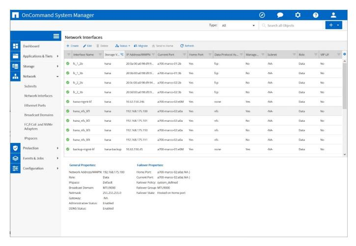
During the SVM creation with ONTAP 9.8 System Manager, you can select all of the required physical FCP ports, and one LIF per physical port is created automatically.
