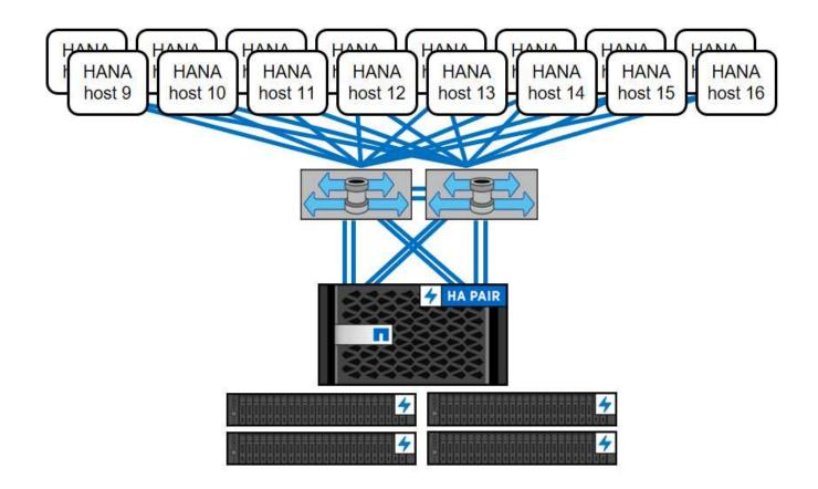
Independent of the deployed AFF system, the SAP HANA landscape can also be scaled by adding any certified storage controllers to meet the desired node density, as shown in the following figure.
