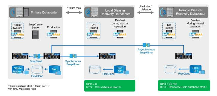
Synchronous replication offers StrictSync mode. If the write to secondary storage is not completed for any reason, the application I/O fails, thereby ensuring that the primary and secondary storage systems are identical. Application I/O to the primary resumes only after the SnapMirror relationship returns to the InSync
