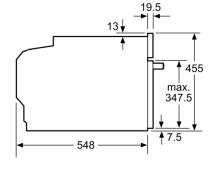
measurements in mm
