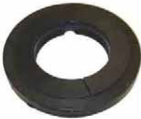
Failed Seal Resulting from Improper Fit
