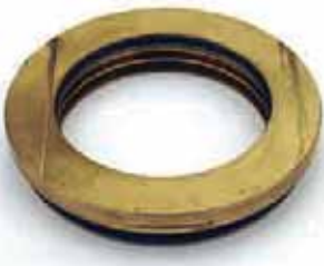
Failed Seal Resulting from Improper Installation
