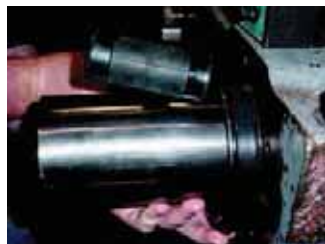
Installing the Seal
