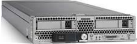
Figure 5 Cisco UCS B200 M4 Blade Server
