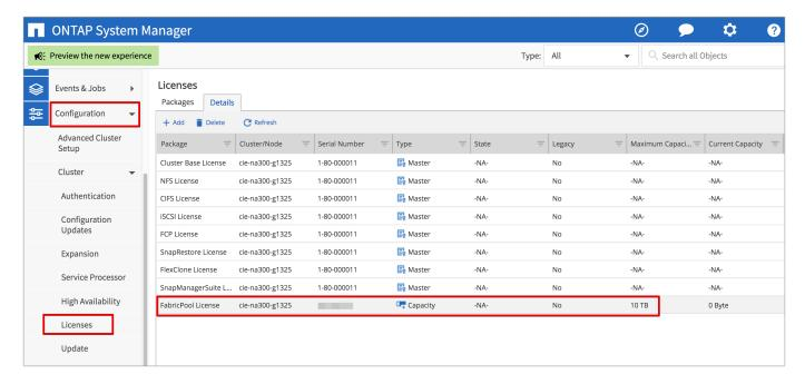
Maximum capacity and current capacity are listed on the FabricPool License row.
