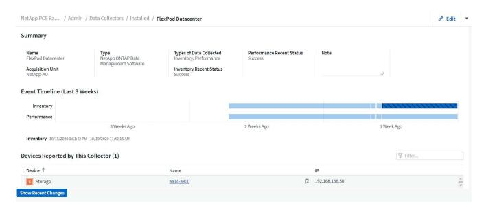
Under the device list near the bottom, click on the name of the ONTAP storage system being monitored. This displays a dashboard of information collected about the system, including the following details:
