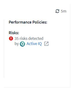
4. To open a new browser tab and take you to the risk mitigation page, which shows which nodes are affected, how critical the risks are, and what the appropriate action is that needs to be taken to correct the identified issues, click the link for Active IQ.
