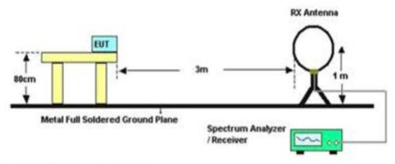
For Radiated Emission 30~1000MHz
