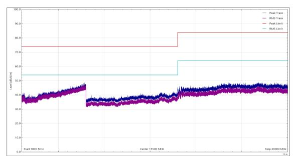
Figure 7 - 1 GHz to 30 GHz, Peak, Horizontal
