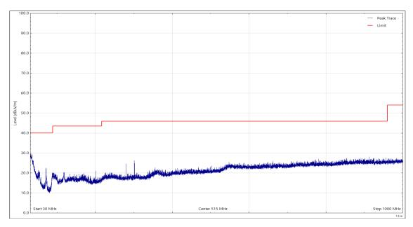
Figure 6 - 30 MHz to 1 GHz, Quasi-Peak, Vertical
