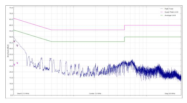
Figure 3 - Graphical Results - AC Power Port Neutral Line
