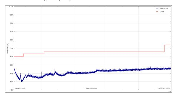
Figure 5 - 30 MHz to 1 GHz, Quasi-Peak, Horizontal
