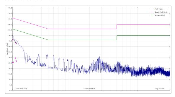
Figure 2 - Graphical Results - AC Power Port Live Line
