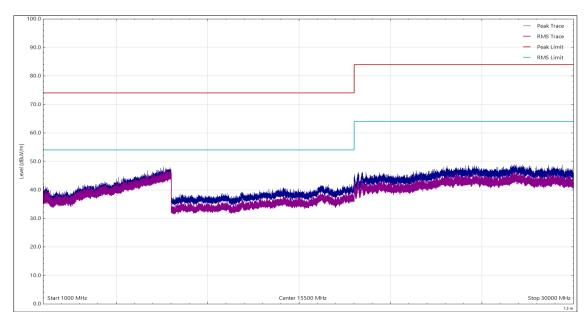
Figure 8 - 1 GHz to 30 GHz, Peak, Vertical
