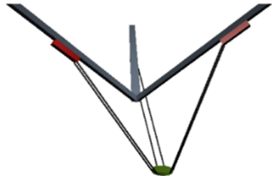
Figure 3. Tripod kinematics with linear axes
