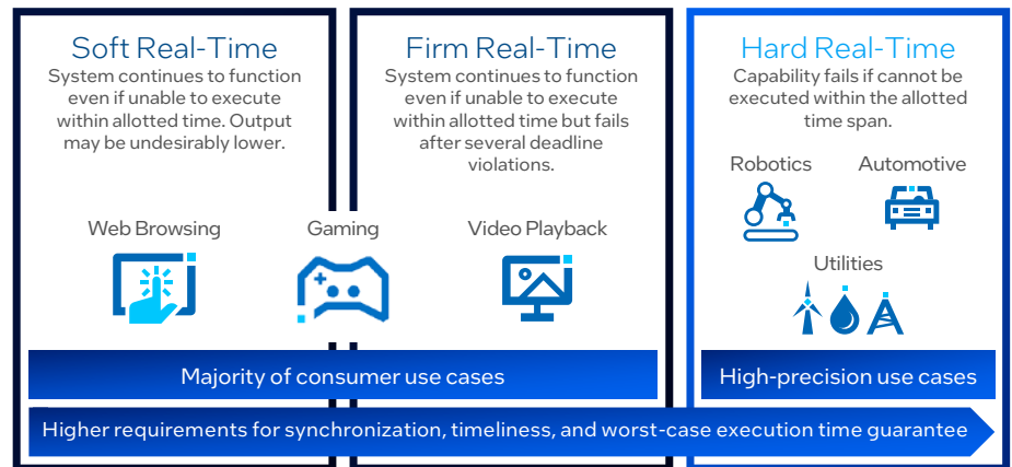
Figure 1. Real-time systems taxonomy: Intel real-time solutions are focused on hard real-time use cases
