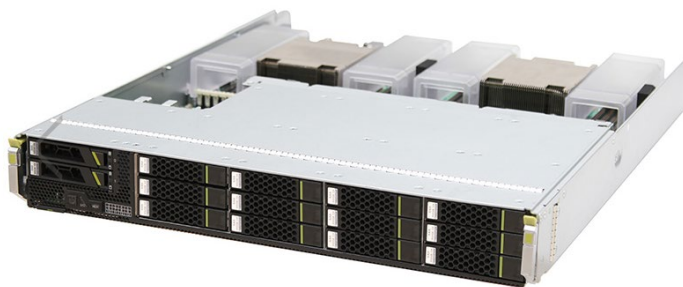
Figure 5-11 CH225 V3 compute and storage node
