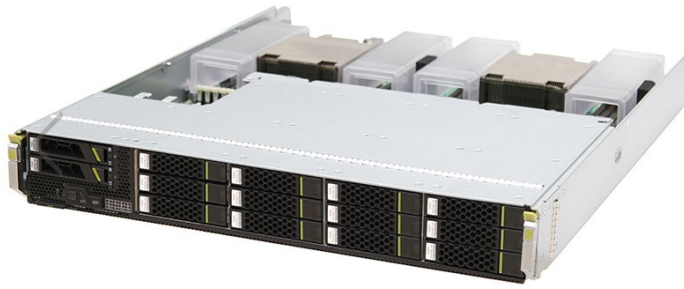
Figure 5-15 CH225 V5 compute and storage node
