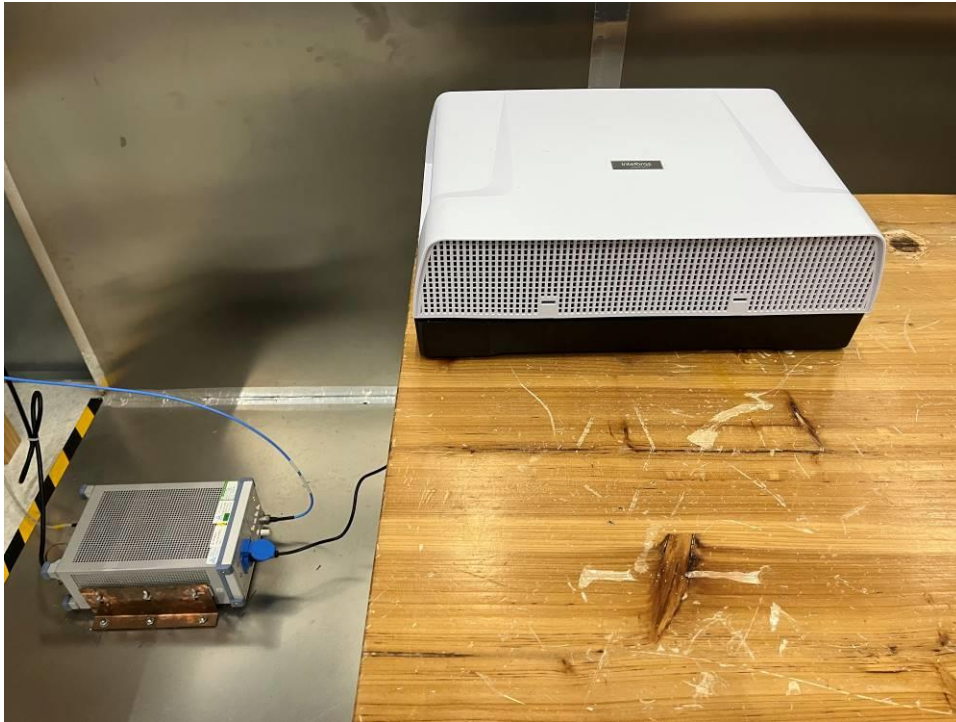
Photograph 1: Set-up for Conducted Emission on AC Mains
