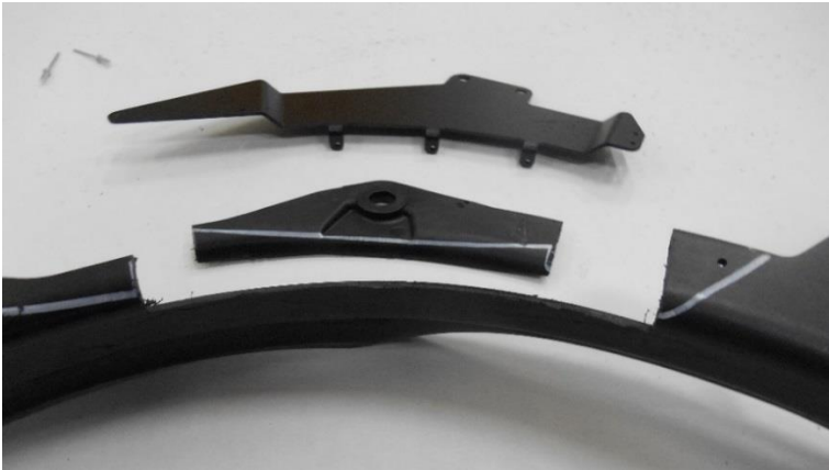
Figure 7 - Modifying the Shroud
