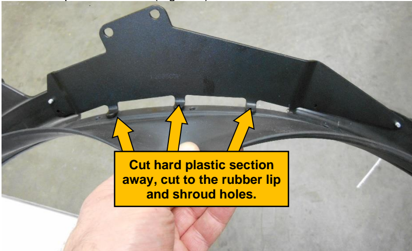
Figure 8 - Modifying the Shroud
