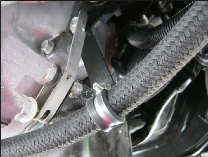
Figure 32 – Securing the hoses
