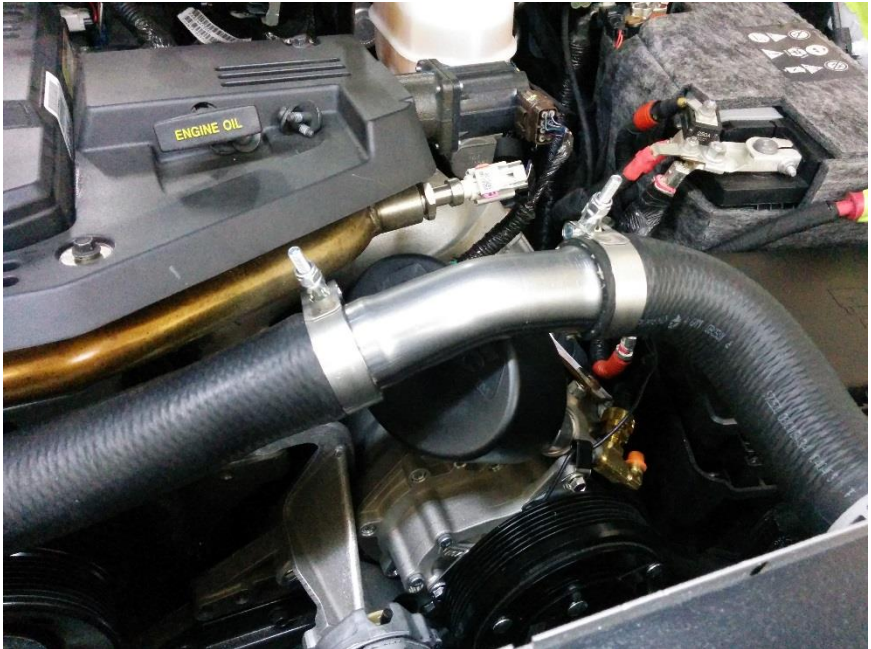
Figure 25 – Connecting the upper radiator hose
