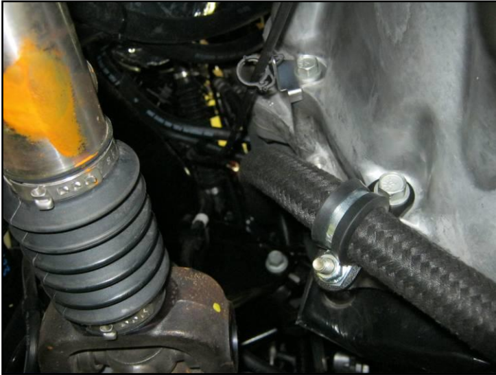
Figure 31 – Securing the hoses
