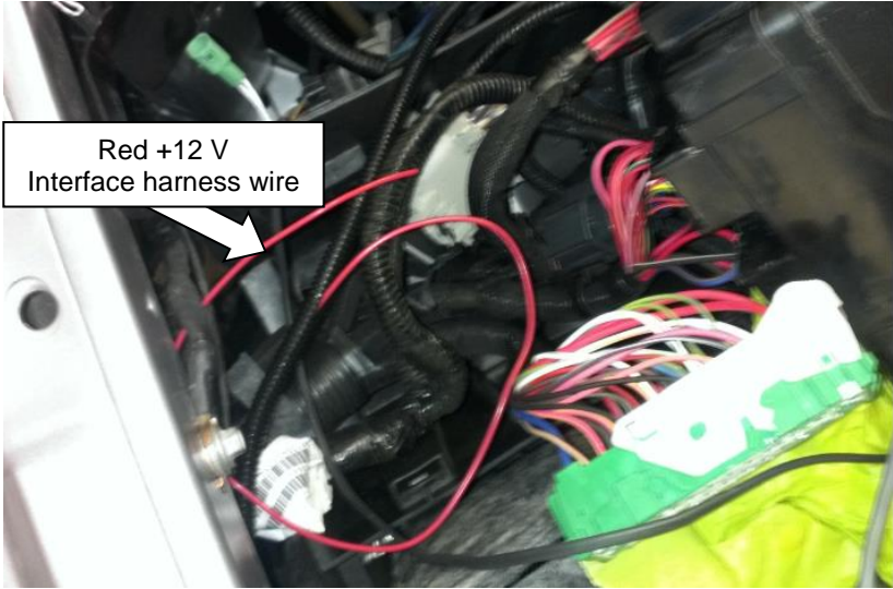
Figure 48 – Connecting to key switched power
