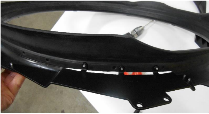
Figure 10 - Stiffener Bracket Attached
