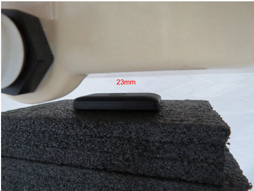
Picture 6: Back Side, the distance from EUT to the bottom of the Phantom is 23mm
