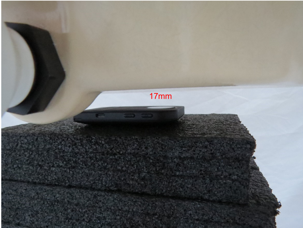
Picture 7: Front Side, the distance from EUT to the bottom of the Phantom is 17mm
