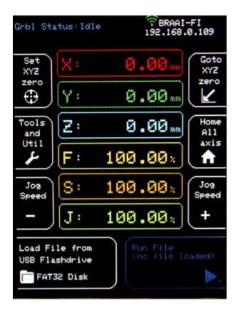
TIP: Adjusting the Jog Speed allows you perform finer grained jog moves for final positioning, the lower the speed, the smaller the distance you can move.
