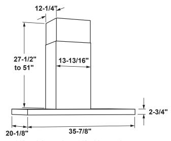
36"models require a 36"-wide opening \*The supplied duct cover fits 7'-7" to 10'-6" ceiling heights (12' ceiling height with optional high celling kit UX12DC9SLSS/UX12DC9BLTS) (14' ceiling height with optional high celling kit UX14DC9SLSS/UX14DC9BLTS)
