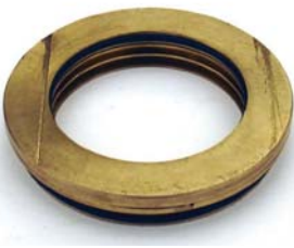
Failed Seal Resulting from Improper Installation
