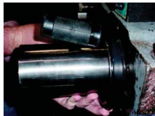
Installing the Seal
