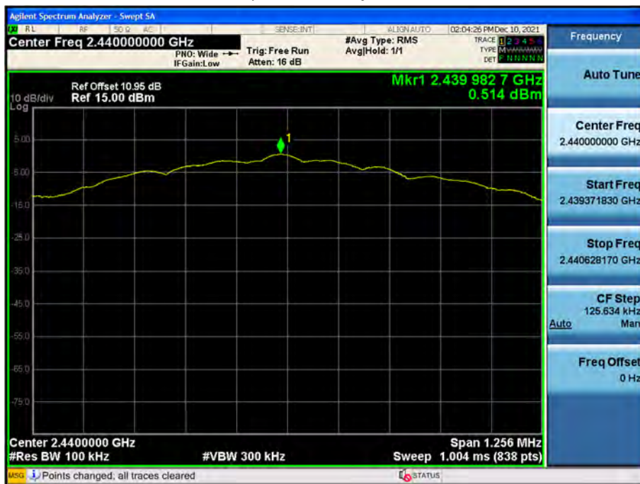
Power Spectral Density (Mid-CH 19)
