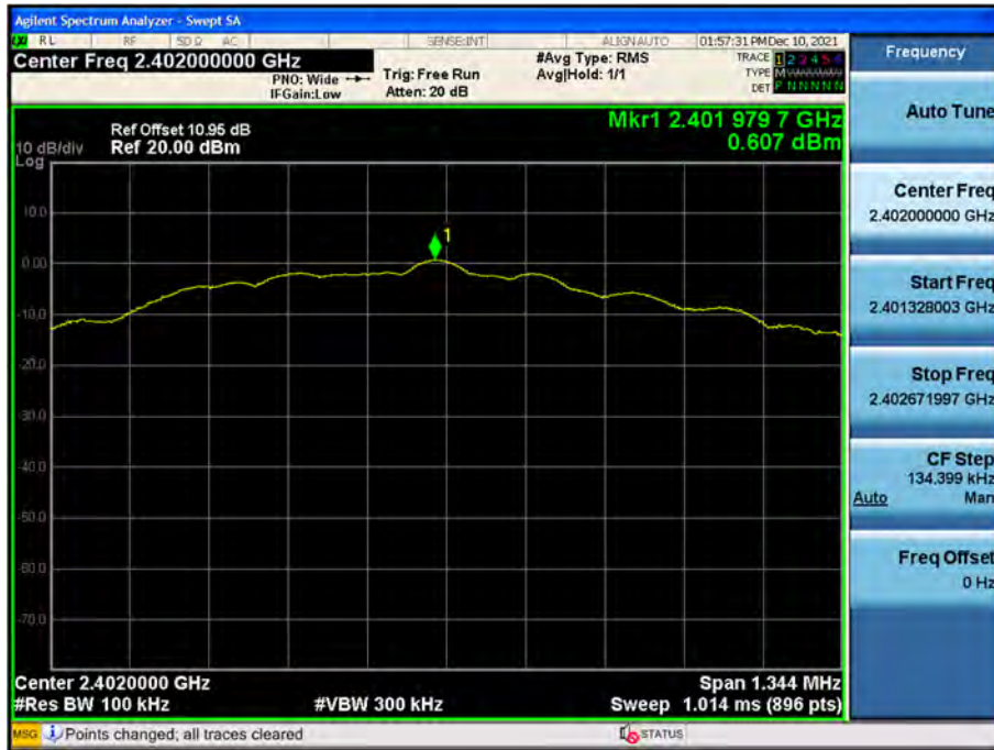
Power Spectral Density (Low-CH 0)
