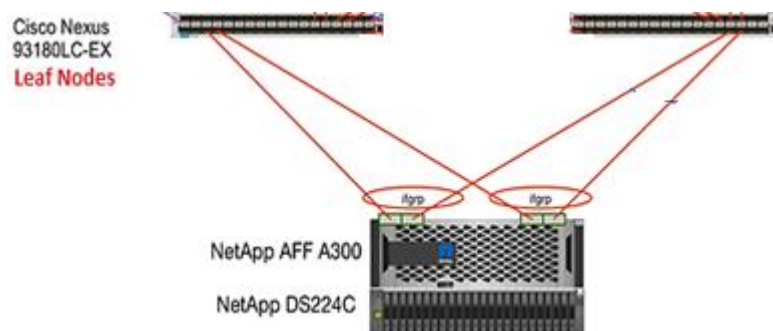
Figure 13 Storage Connectivity to ACI Leaf Switches
