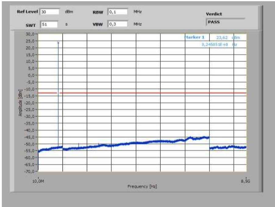
Plot 7: Lowest Channel (10 MHz – 8.5 GHz), spacing 15 kHz, 1@0 tones
