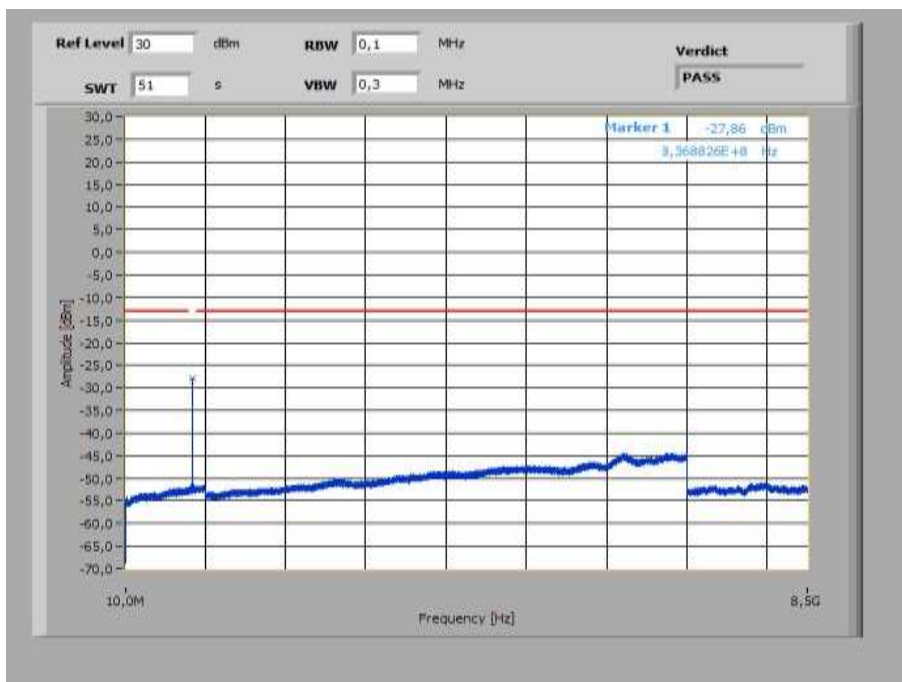
Plot 8: Middle Channel (10 MHz – 8.5 GHz), spacing 15 kHz, 1@0 tones
