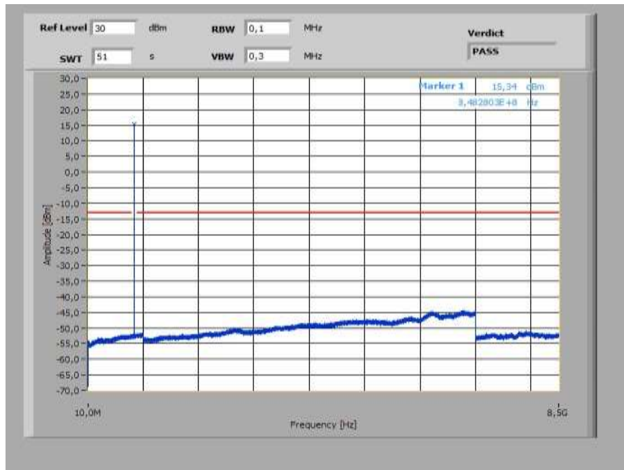
Plot 15: Highest Channel (10 MHz – 8.5 GHz), spacing 15 kHz, 12@0 tones
