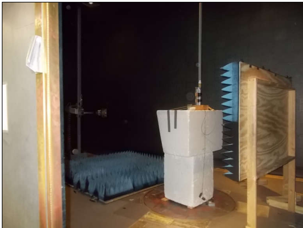
Figure 2: Radiated Emissions – YPOS
