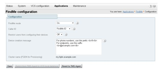
The picture below shows example usage of the FindMe Express end-user interface. In particular it shows how the **Device creation message** may appear when a user is specifying a new device to add to their Findme profile.
