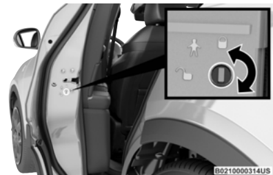
Child-Protection Door Lock Function
