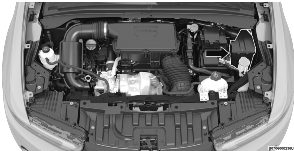
Underhood Power Distribution Location
