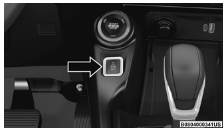
Stop/Start OFF Switch
