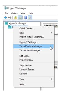
2. If the virtual switch containing the name of the network adapter used in this product is displayed in **Virtual Switch** on the left pane, select it and change the settings below.
