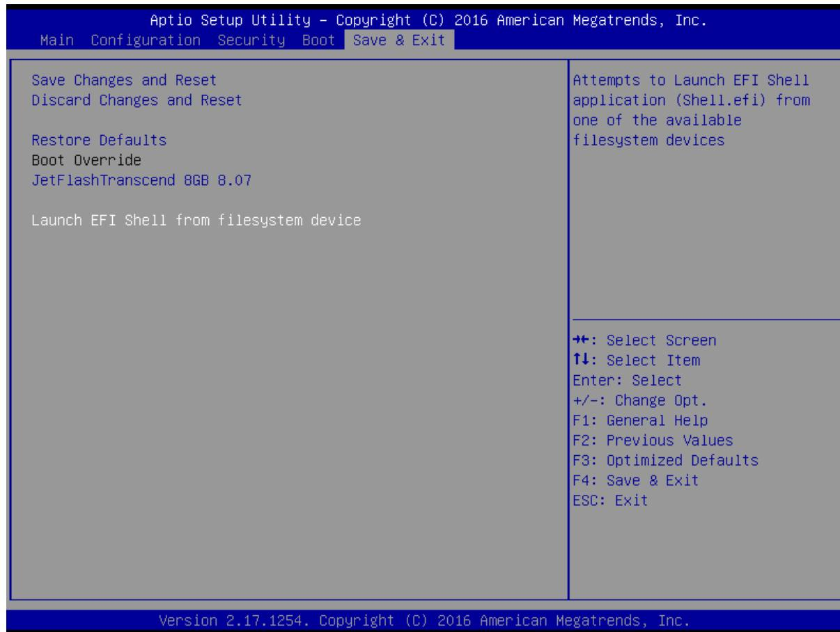
Step 5. Under the UEFI shell, direct to your USB DOK, below is an example uses fs0. Then direct to the folder with updated file and type command : "update" and press enter.
